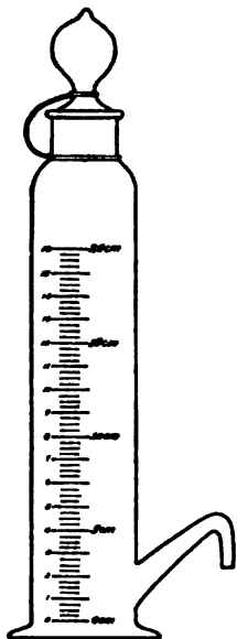
FIG. 14. — Atterberg's silt cylinder for the mechanical analysis of soil by subsidence.
